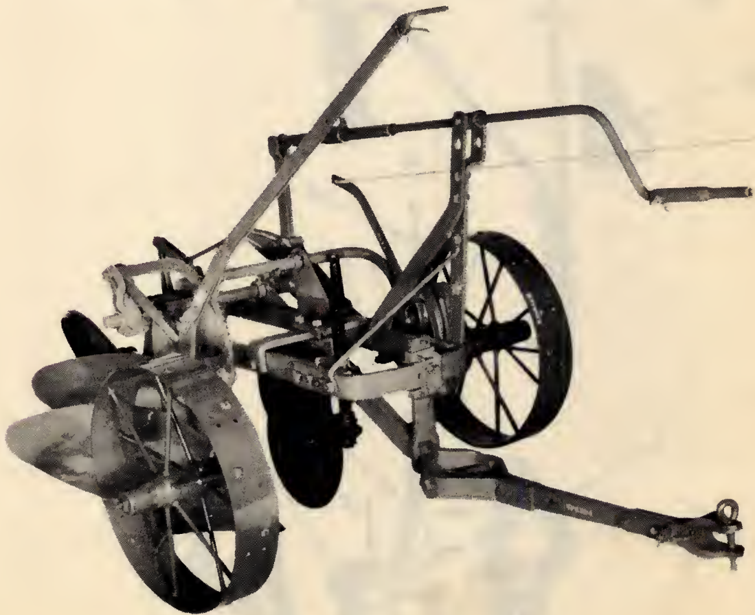
FIGURE 3 No. 216 Tractor Gang Plow Equipped with Wide Tire Steel Wheels, Row Crop Depth Adjusting Screw, Draw Bar Extension, Screw Extension and Break Pin Clevis
