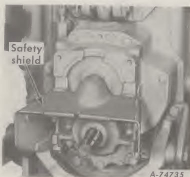
Illust. 50 Safety shield in place for 540 r.p.m. Power take-off.
