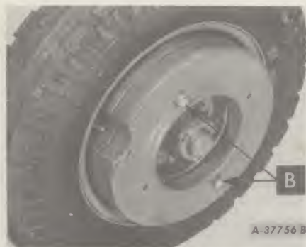
Illust. 96A First and second front wheel weights assembled on the tractor.
