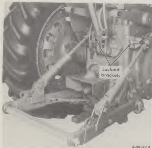
Illust. 48 Connecting the lift links to the lockout brackets.
