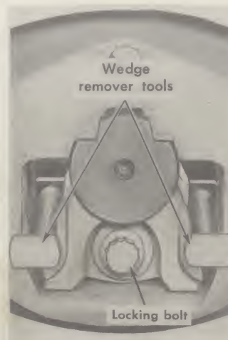
Illust. 90B Tools in place with offset head over wheel hub face.
