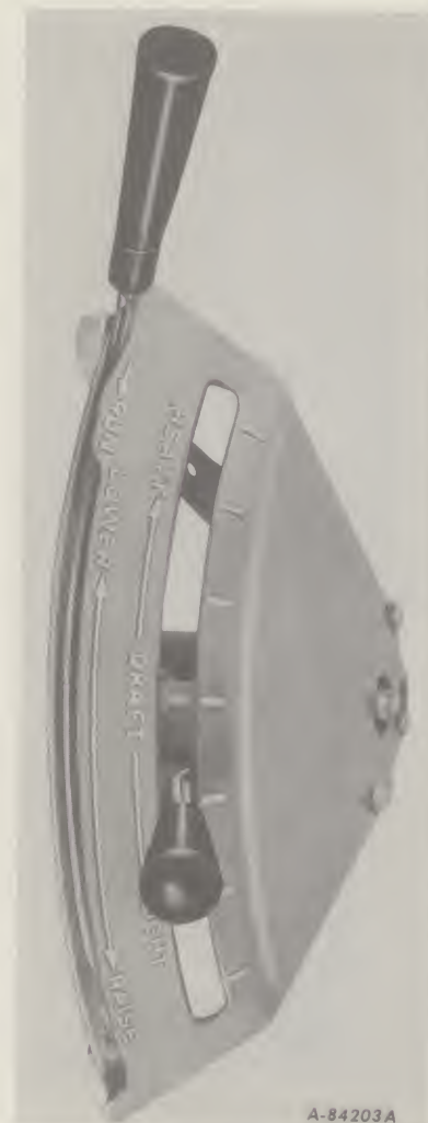
Illustr. 30A Inside control lever set for slow draft sensing response.
