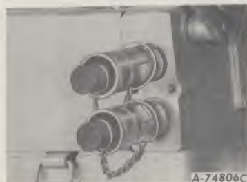
Illust. 43 Rear junction ports operated by the inner or single control lever.
