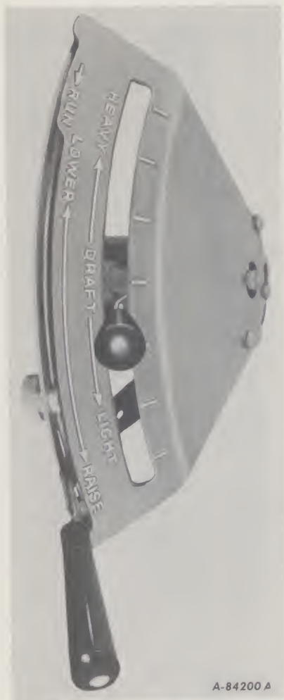
Illust. 29 Inside control lever used to raise the equipment without moving the draft control lever.
