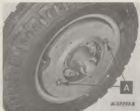
Illust. 96 First front wheel weight assembled on the tractor.
