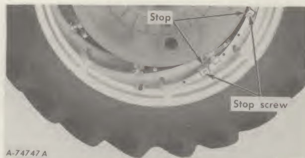
Illust. 94A Position of stop before power-adjusting the rim.
