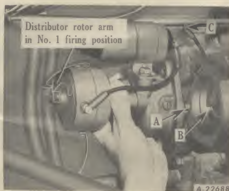
Illust. 6 - Assembling the battery ignition unit on Farmall Super-A. Other models are similar.
